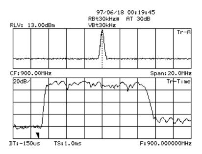
Figure 6. Split-screen frequency domain and time domain displays.
