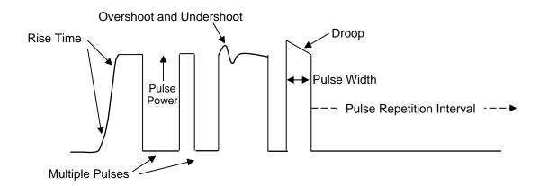
Figure 3. Important time domain characteristics of radar signals.
