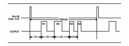
Figure 5. Quad pulse with spectrum analyzer trigger signal.
